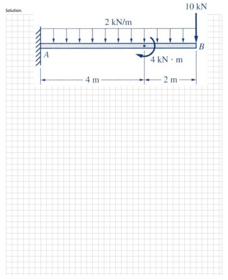
3-56 See Fig. P3-56. Determine the reactions at supports A and B due to the applied loads shown.
